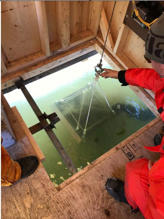
b) Diver box deployed from hoisting hut on the ice cover with support from professional divers
